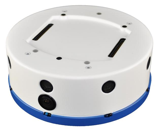
The Khepera IV is the perfect platform for the indoor research with a single robot or in swarm in a limited space such as a Lab floor or a table top. Highly modular, it accepts various options to adapt the robot to your application.
