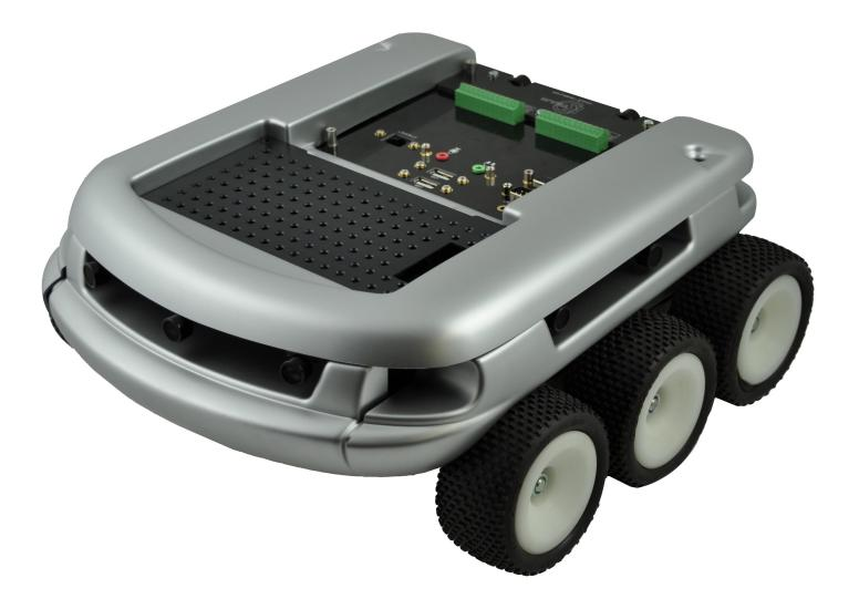
The Koala is a mid-size robot designed for real-world applications. Bigger than the Khepera, more powerful, and capable of carrying larger accessories, the Koala has the necessary functionalities for use in practical applications (like navigation, mapping, artificial intelligence, ...), it rides on 6 wheels for indoor or outdoor all-terrain operation, with a sports stylish bodywork for attractive demonstrations.
