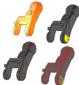
**Integrated edit modes:** e.g. mesh edit modes, including a semi-automatic primitive shape extraction method (invaluable to create scenes with optimized dynamic content)
