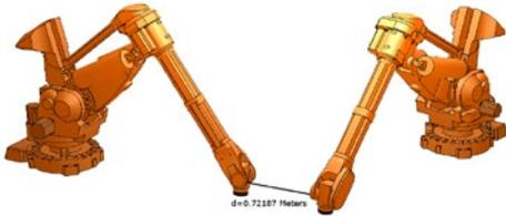
**Collision detection and distance calculation:** Fast interference checking and minimum distance calculation between any meshes or collection of meshes
