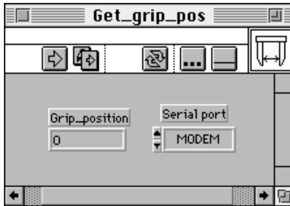
Figure 11: Get_grip_pos panel: a display indicates the position of the gripper.
