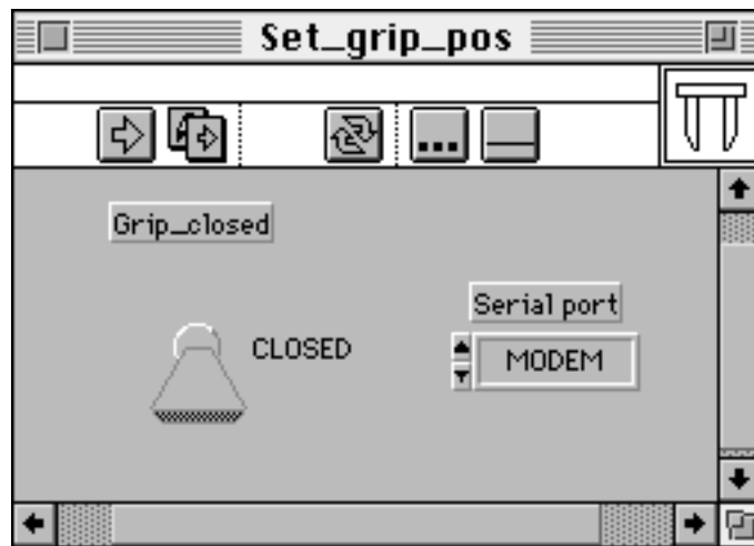
Figure 10: Set_grip_pos panel: a switch allows to open or close the gripper.
