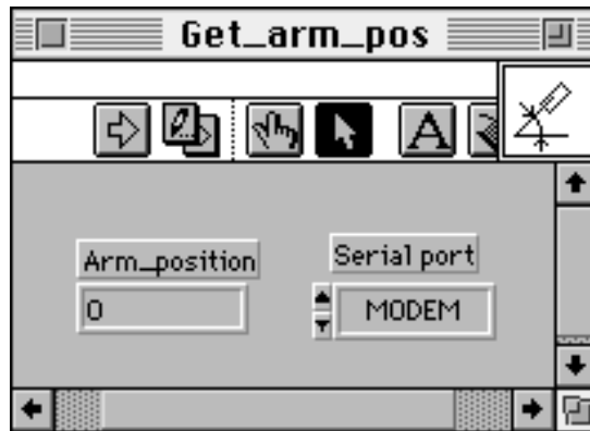
Figure 9: Get_arm_pos panel: a display indicates the position of the arm.
