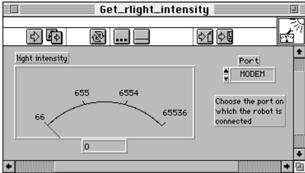
Figure 9: This instrument indicates the light intensity in the field of view of the K213 vision turret.
