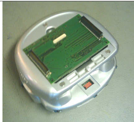
6) Insert the upper part of the Korebot II
