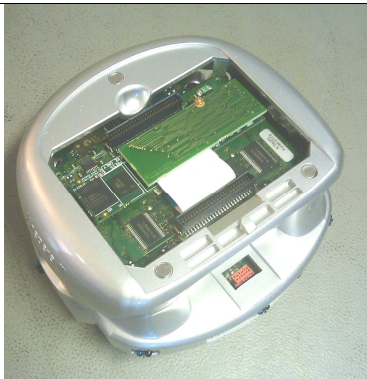
5) Put the cover of the Khepera III and rescrew it
