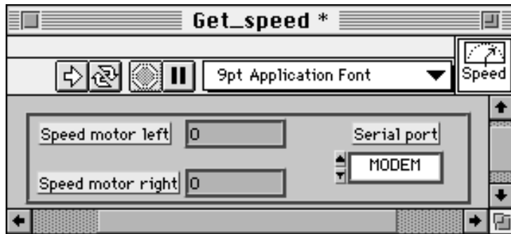
Figure 21: Get_speed panel: 2 indicators show the speed of each wheel.
