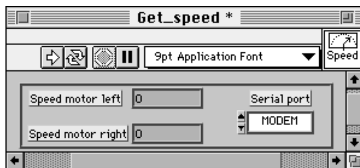
Figure 21: Get_speed panel: 2 indicators show the speed of each wheel.
