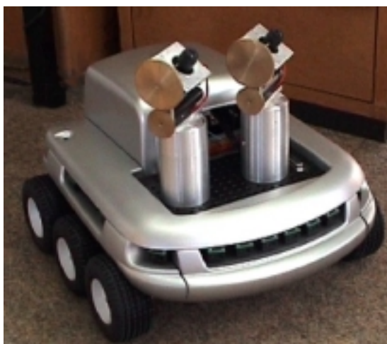
Figure 1a (left) – Double Pan-Tilt Camera mounted on Koala robot Figure 1b (right) – REB motor ports 0 and 1
