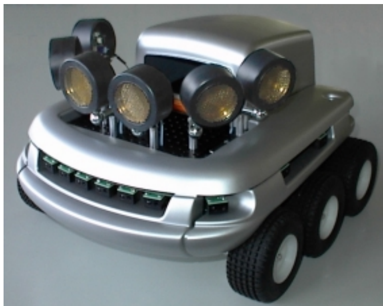
Figure 1 - Koala equipped with 6 sonar sensors
