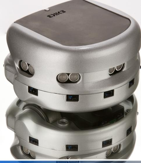
The Khepera III is a real concentrate of technologies. It has the same performances of much bigger robots but can be hold in one hand. The Khepera III is designed to perform complex individual or swarm applications in a limited space such as a table top or on your lab floor. The possibilities are almost unlimited with all the extensions available, making it a standard in many worldwide universities.
