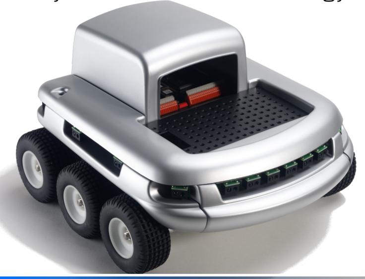
The Koala robot is a robotic platform for real-world experiments and full-scale demonstrations. Fully software compatible with Khepera, it has been designed to be easy to use, easy to transport and able to deal with a standard office environment as well as a rough indoor terrain. The possibilities are almost unlimited with all the extensions available, making it a standard in many worldwide universities.
